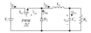
2. (10%) If the following converter operates in CCM, please sketch in turn the waveforms of PWM (=  $v_{gs}$ ),  $i_{ds}$ ,  $i_{Do}$ ,  $v_{Do}$ ,  $i_{Co}$ ,  $v_{Co}$ .
