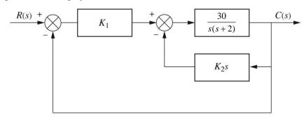
10% (a) Find the equivalent transfer function C(s)/R(s).
