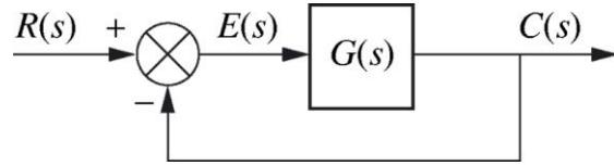
4. (20%) Design the  $K$  value to yield 0.1% error in the steady state for the following system.
